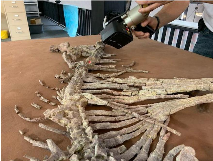
**NVision's non-contact HandHeld scanner is ideal for capturing the geometry of fragile objects, such as the nearly 300-million-year-old Dimetrodon skeleton**
