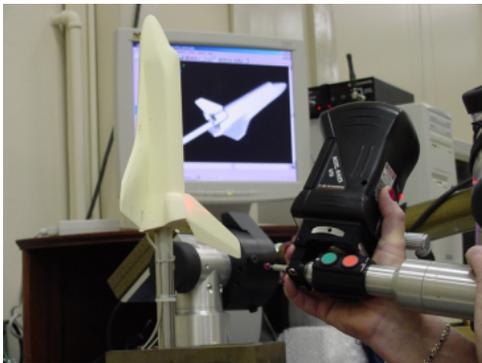
NVision's versatile HandHeld scanner is capable of capturing 3D geometry from objects of almost any size or shape.
