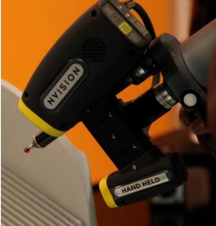
**NVision's HandHeld scanner, shown in a different application, rapidly collects massive amounts of individual location points on an object's surface.**
